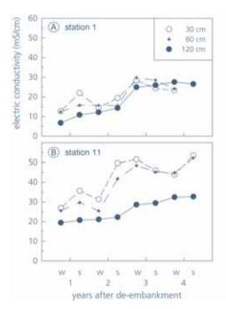
Figure 3. Increase of the EC value of the groundwater in the trial saltmarsh near the dike breaches in the western (Location 1) and eastern parts (Location 11), during the first four years after the de-embankment.
